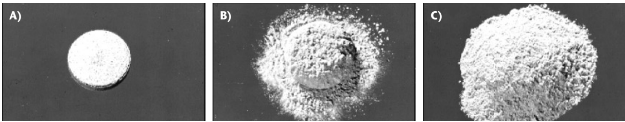
Figure 1. Tablets of aluminum phosphide. A) Just placed. B) Reaction to phosphine release. C) Phosphine completely released.
